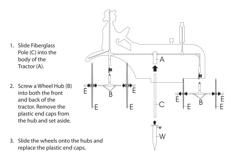
**NOTE:** For use in high winds and for extra durability we recommend applying epoxy glue in the end caps.
